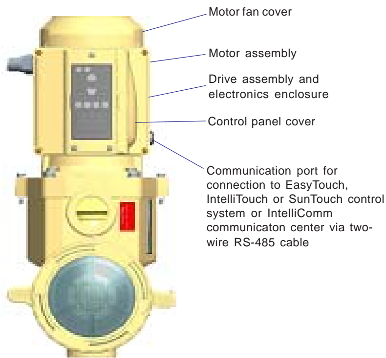
IntelliFlo VS-3050 Motor Assembly
